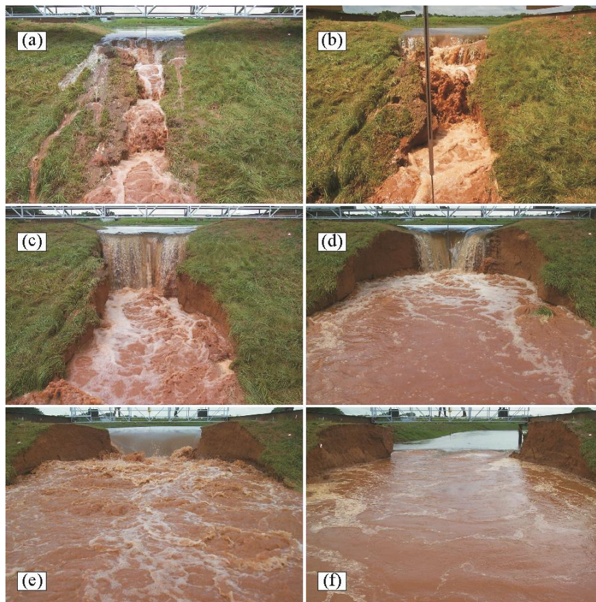
Fig. 2.5. Cohesive dam breaching by overtopping: (a) rills and cascade of small overfalls at t=7 min; (b) consolidation of small overfalls at t=13 min; (c) headcut at downstream crest at t=16 min; (d) headcut at upstream crest at t=31 min; (e) flow through breach at t=40 min; (f) transition to final breach stage at t=51 min (Experiment by Hanson et al., 2005)
