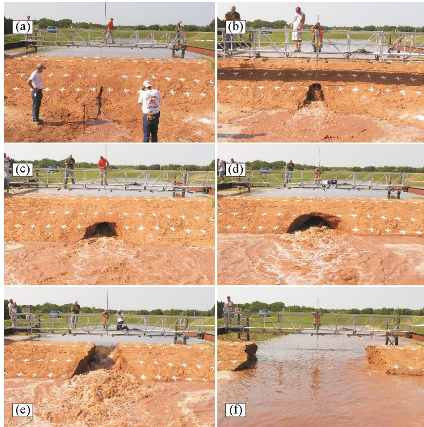
Fig. 2.14. Dam breaching due to piping: (a) initiation; (b) t=5 min; (c) 8 min; (d) 13 min; (e) 13 min, following collapse of piping roof; (f) 60 min, continued widening (Experiment by Hanson et al., 2010)
